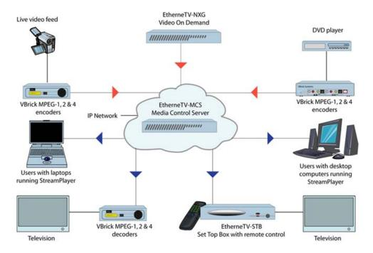
Figure 1. EtherneTV Media Distribution System
